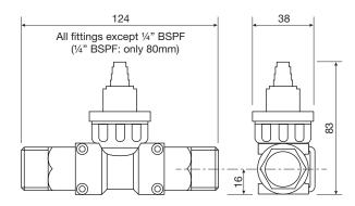
This multi-range radial flow turbine meter uses a low inertia turbine supported on robust sapphire bearings in a chemically resistant housing. Nine flow ranges (0.02 to 160 L/min), a choice of 'plug in' fittings and individual traceable calibration, make this meter one of the most flexible available.
