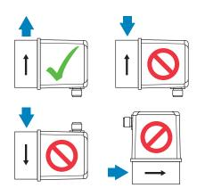
Observe direction of flow arrow on steel body
