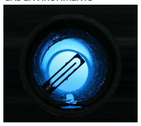
Kurz thermal mass flow meters provide excellent measurement capabilities in dry gas flows. They have proven durability, accuracy, and repeatability. Where all thermal meters have been largely ignored is in the biogas environment. Condensation levels in biogas fluctuate as temperatures change during the day, and it's the highly unreliable readings from those liquid droplets vaporizing on the sensors that make wastewater and landfill operators dismiss thermal meters.
