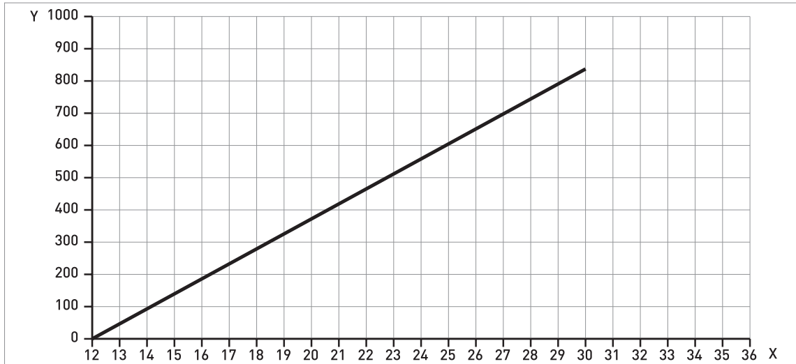
Figure 2-9: Minimum power supply voltage for an output of 21.5 mA at the terminals (Non-Ex and Hazardous Location approval (Ex i / IS))
