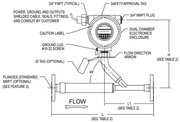
DIRECTLY ATTACHED ELECTRONICS ENCLOSURE (TA)
