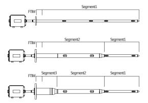
**Note:** The additional material used to increase the diameter of segments 2 and 3 also slows the effects of corrosion on the probe support.
