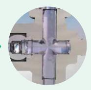
Then open the bottom valve to the bypass position. Fluid will now flow through the valve and into the glass without seating the ballcheck.
