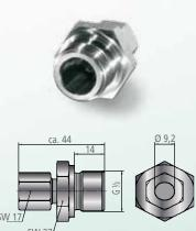
Through-bolt joint item no. 532 160 For gas-tight mounting in tubes and channels; atmospheric pressure Material: Stainless steel 1,4571, clamping ring PTFE
