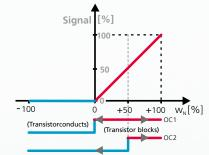
Remark: in an unidirectional design, the switching output OC1 is used as flow indicator by default (configurable). It will clearly show a flow higher than 0 m/s by blocking and will switch if this is less or equal to 0 m/s. Arrows in the representation of the switching outputs mean that the threshold value can be configurated. The factory setting for the switching output OC2 is 50 % of the measurement range (option: customer-specific switch point).
